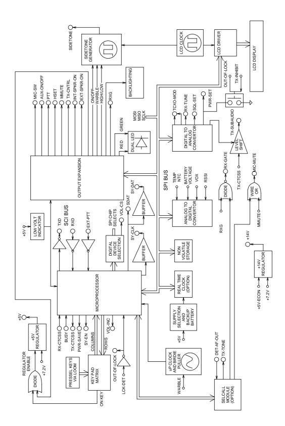
Figure 2.2 T3010 Control PCB Block Diagram
